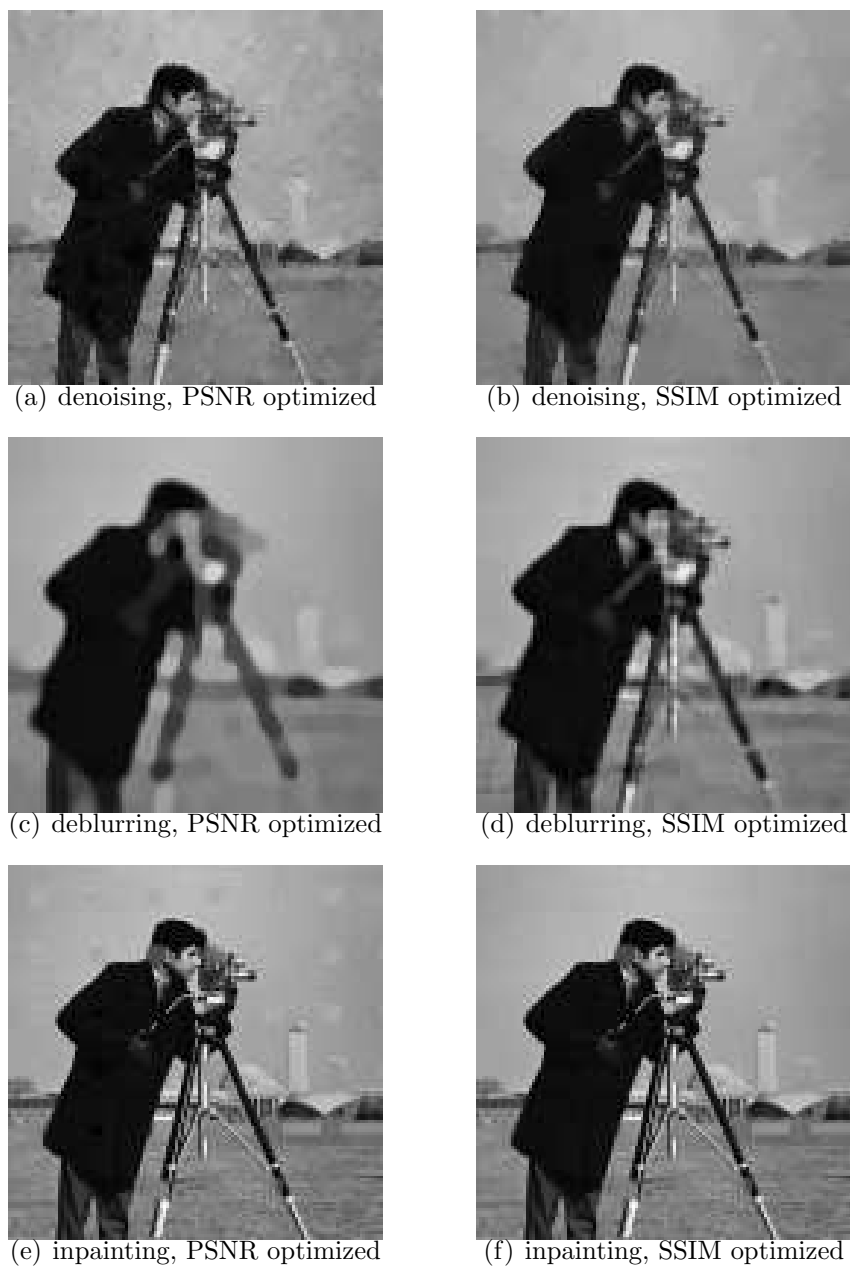
Figure 8.27: Influence of quality measure on automated parameter selection: We consider the applications of denoising, deblurring and inpainting on the cameraman image and focus on standard TV regularization. We optimize the parameter \alpha of the TV regularizer by a hierarchical grid search using the PSNR (left column) and the SSIM index (right column). Obviously the SSIM index is the more suitable quality measure for the task of finding optimal parameters.
