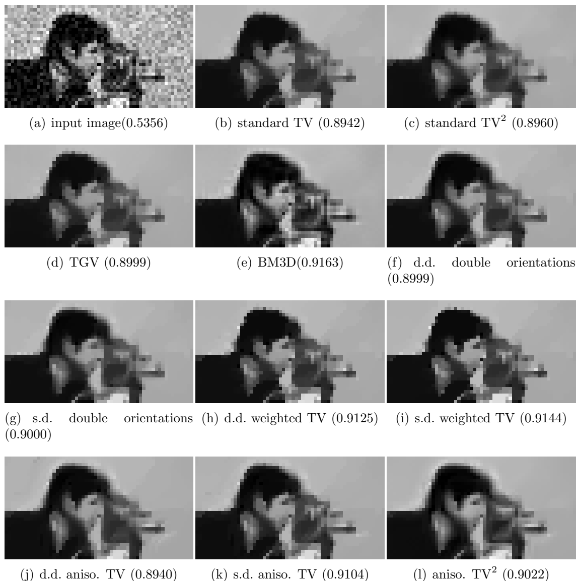
Figure 8.3: Denoising of the cameraman image. Qualitative comparison of the considered denoising methods on a close-up of the head region of the cameraman image. (For the sake of completeness, we provide the SSIM indices, now determined on the specific image region. The PSNR gives the same ranking.) BM3D [47] also in terms of visual appearance provides the best result. Weighted TV produces an almost as sharp result as BM3D. The other methods produce smoother results.
