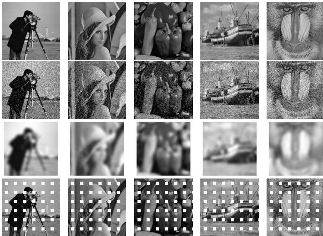
Figure 8.1: Test images used to evaluate adaptive TV regularization for the applications of denoising (2nd row), deblurring (3rd row) and inpainting (4th row). The first row shows the original undistorted images. For the application of deblurring, due to the support of kernel function, the data are given only on \Omega_f \subseteq \Omega . In the test images for inpainting the regions colored in white indicate the regions to be inpainted.
