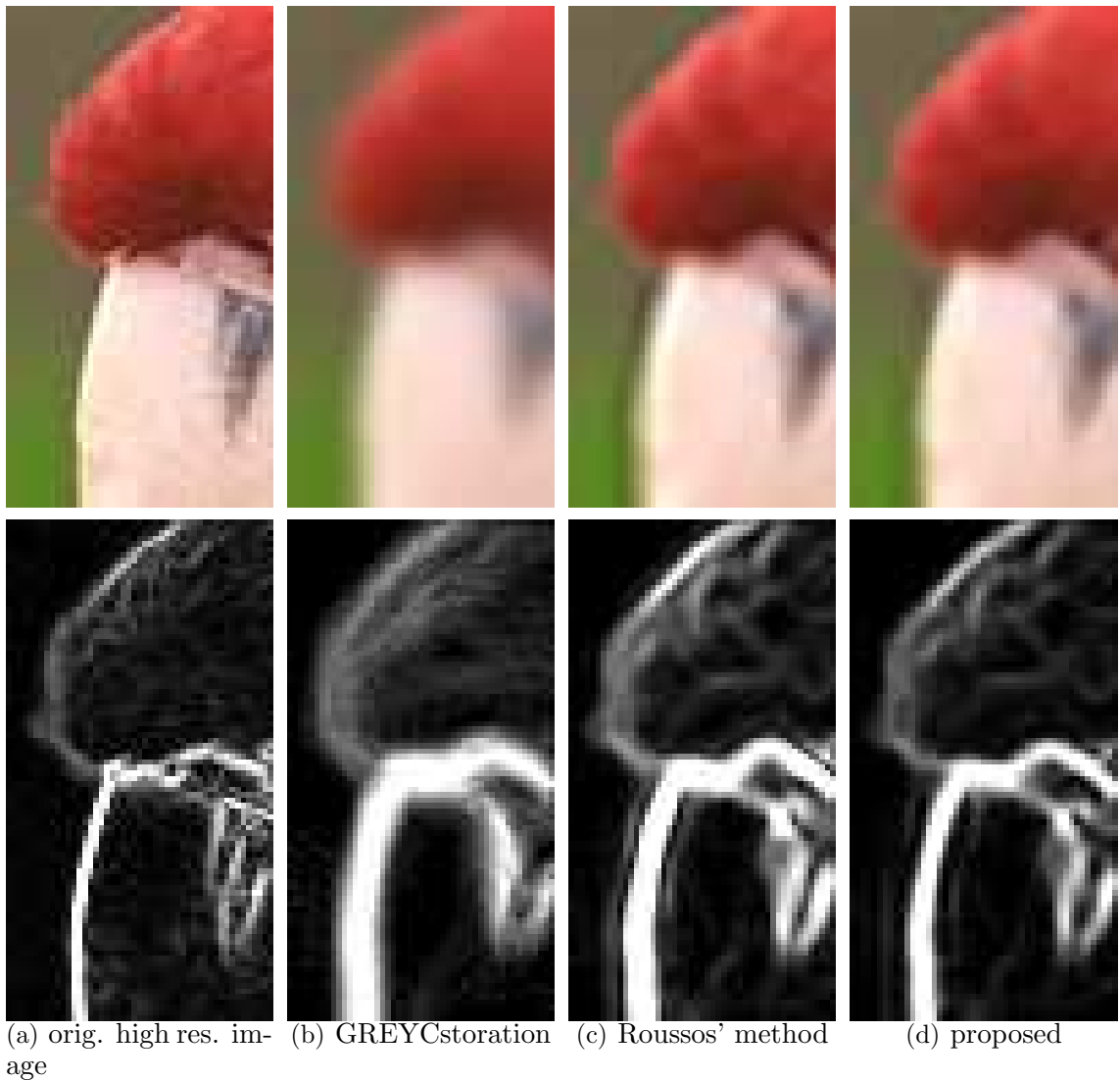
Figure 8.50: [Best viewed in color.] Top row: detail of an edge in the original high resolution image (a) and interpolated images, using GREYCstoration with interpolation constraints (b), Roussos' method (c), and the proposed method (d). Bottom row: results of subsequently applying the Sobel operator to the interpolated images. The proposed method provides the sharpest and most regular reconstruction of the edge.
